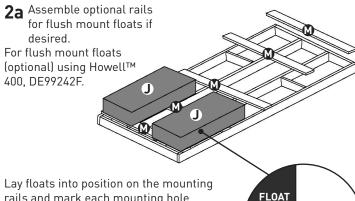
rails and mark each mounting hole location. Drill 3/16" pilot holes at each location to be used.
