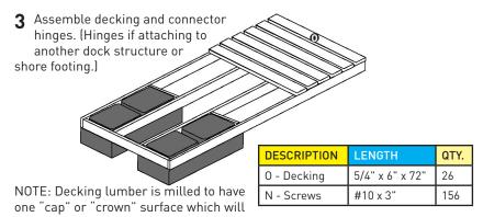
allow water to flow away from the deck surface. When mounting the deck boards to the dock frame it is recommended to fasten the decking "cap"/ "crown" up.
