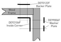
Always use washer plates (DE99006F), backer plate (DE93122F) or mating hardware components together. Farmework of the dock structure should be sandwiched between hardware pieces at all joint locations as shown.
