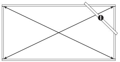
2 Lay the dock frame upside down on a flat surface in order to easily install floats.
